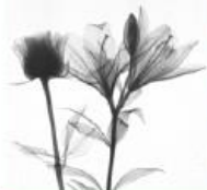
Neutron Radiography (Panel exhibition) Neutron radiography can visualize water or oil inside materials
